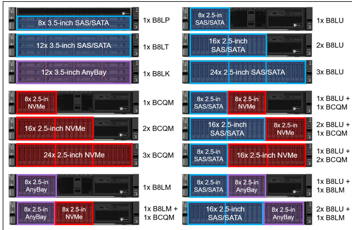
Figure 7. SR665 front drive bay configurations
